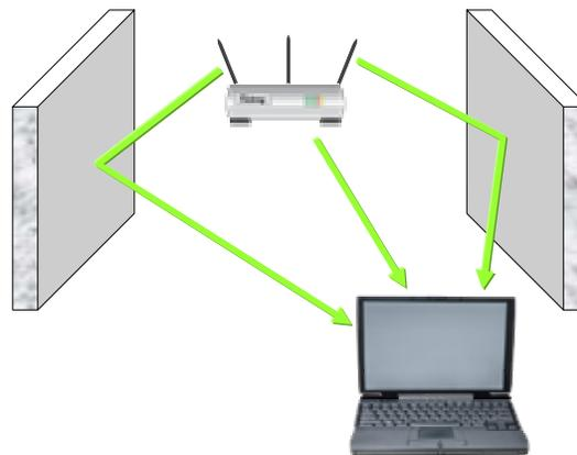
Aside from spatial multiplexing, 802.11n devices can also use the traditional styles of receiver spatial diversity, such as Maximum Ratio Combining (MRC). The standard also introduces transmitter spatial diversity techniques, such as Space Time Block Coding (STBC) and Cyclic Shift Diversity (CSD), to improve reception by spreading the spatial
