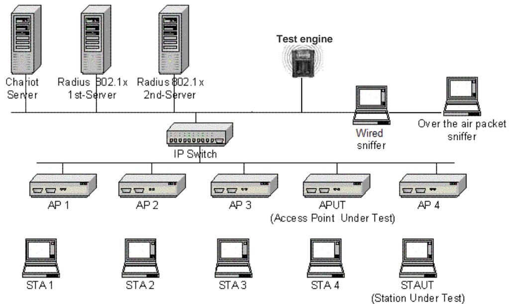
**Fig 2: Typical over-the-air certification test bed tests a client against 4 APs or an AP against 4 clients. Devices in the test bed are based on silicon from different vendors.**
